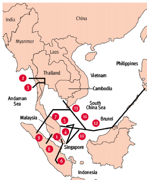
Fig. 2. The Proposed Trans-ASEAN Gas Pipeline (TAGP) Network. Source: modified from Peter Roberts and Alex Cull, “Building the Trans-ASEAN Gas Pipeline,” Asia Pacific Review (July, 2003), pp. 15–20. Legend: (1) Malaysia to Singapore, (2) Myanmar (Yadana) to Thailand (Ratchaburi), (3) Myanmar (Yetagun) to Thailand (Ratchaburi), (4) Indonesia (West Natuna) to Singapore, (5) Indonesia (West Natuna) to Malaysia (Duyong), (6) Indonesia (Grissik) to Singapore, (7) Thailand (Joint Development Area) to Malaysia, (8) Indonesia (South Sumatra) to Malaysia, (9) Indonesia (Arun) to Malaysia (commissioning estimated 2010), (10) Indonesia (East Natuna and West Natuna) to Malaysia (Kerteh) and Singapore (commissioning estimated 2010), (11) Indonesia (East Natuna) to Thailand (JDA-Erawan) (commissioning estimated 2012), (12) Indonesia (East Natuna) to Malaysia (Sabah) and the Philippines (Palawan-Luzon) (commissioning estimated 2015), and (13) Malaysia-Thailand (JDA) to Vietnam (Block B) (commissioning estimated 2016).
